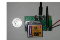
Figure 4: Possible embodiment of a device dedicated to playback vibrations to termites, based on the Gumstix, embedded computer platform.
