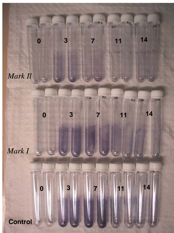
Fig 3. Established biofilms of Pseudomonas aeruginosa in tap water. Biofilm growth was checked at Day 0, 3, 7, 11 and 14. Duplicate tubes were stained biofilm formation using crystal violet.
